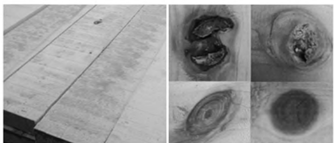
图4 杉木锯材材色样本的实物图 Fig.4 Samples of sawn timber with different colors
